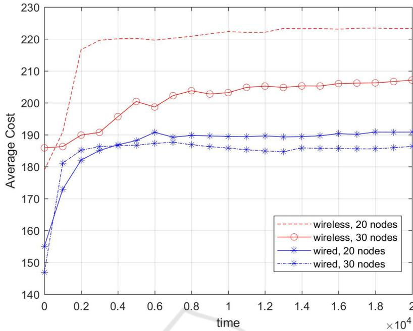
Figure 3: Average Cost in Wireless(With The Extended Model) and Wired Networks(With The Basic Model) with Increasing Number of Nodes.
