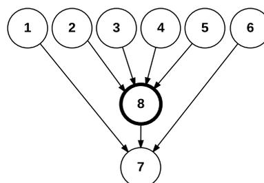
Figure 4: Part of Bayesian network of Pump P-0701 Shutdown after divorcing node method.
