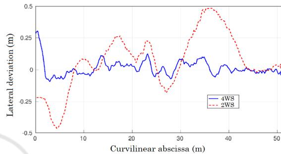
Figure 4: Comparison of tracking errors with and without the use of rear steering angle.
