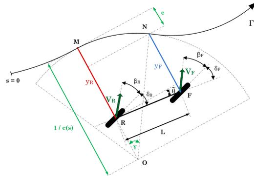
Figure 1: Extended kinematic model of the robot with respect to the reference trajectory  $\Gamma$ .
