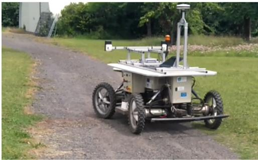
Figure 2: Experimental robot and on-boarded sensor.
