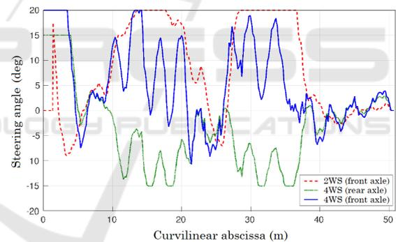
Figure 5: Comparison of front steering angles, and rear steering angle when used.
