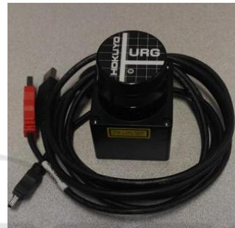
Figure 1: URG-04LX laser sensor manufactured by Hokuyo.
