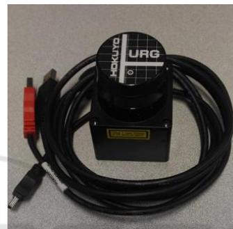
Figure 1: URG-04LX laser sensor manufactured by Hokuyo.
