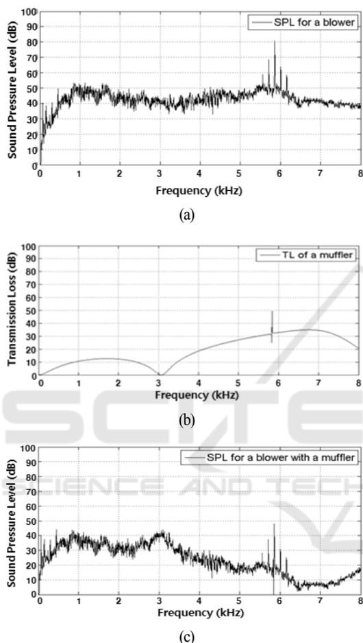
Figure 10: (a) blower noise spectrum, (b) TL of the designed perforated muffler and (c) reduced noise spectrum.
