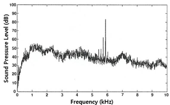
Figure 4: Noise spectrum of a regenerative blower.
