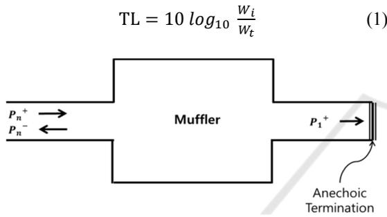
Figure 5: Layout for transmission loss.
