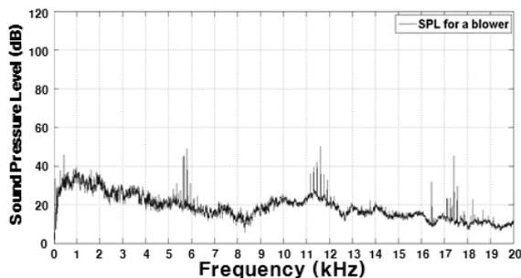
Figure 14: Noise spectrum of regenerative blower with attached perforated diffusive muffler.
