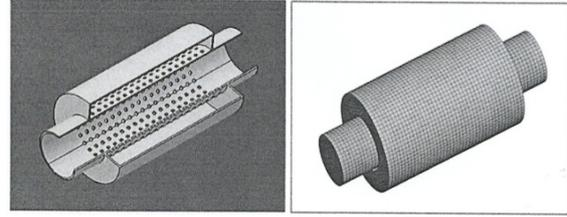
Figure 8: Structural shape and finite element model of a muffler.
