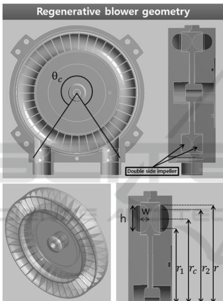
Figure 1: Geometry and design variables of regenerative blower.
