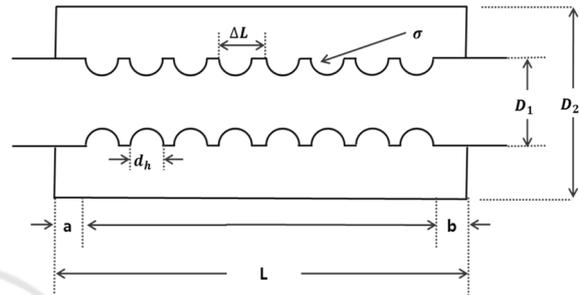
Figure 7: Perforated muffler.
