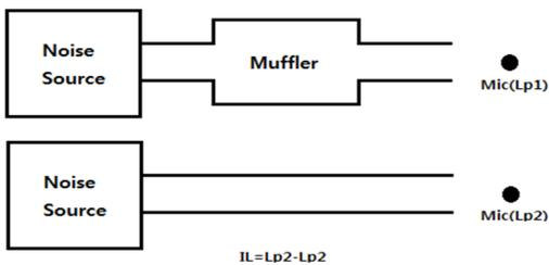
Figure 6: Layout for insertion loss.
