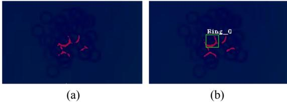
Figure 8: A case with an inclined object, (a) Object detector does not detect the object (b) After increasing the depth threshold, the object detector detects the object.
