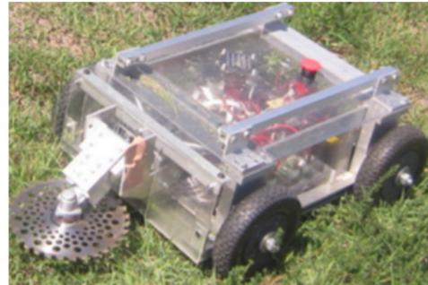
Figure 1: Photograph of the mower robot AMR-D01.
