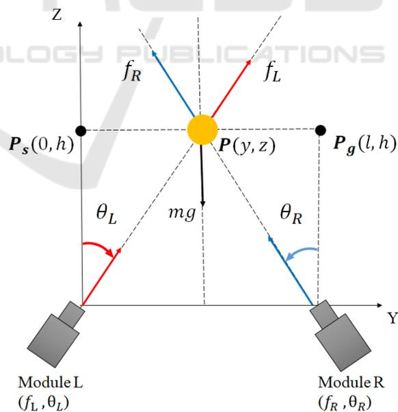
Figure3: Configuration of the experiment system (The angle is positive for clockwise rotation).
