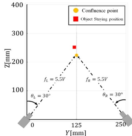
Figure 4: Position of the levitated object and confluence point of the two air jets.
