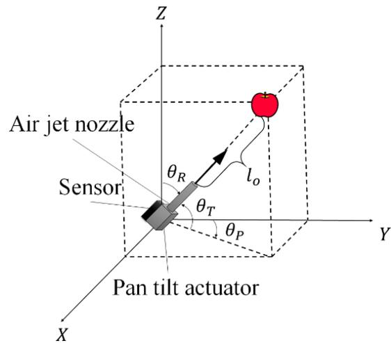
Figure 1: Configuration of "one nozzle control module".
