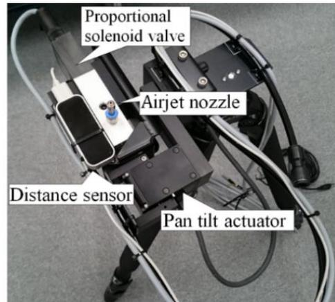
Figure 6: An overview of "one nozzle control module".
