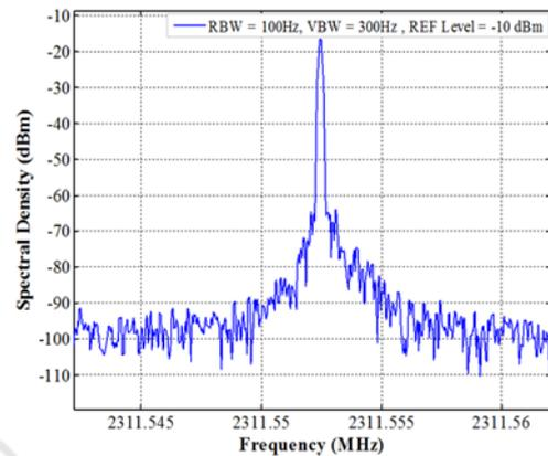
Figure 5: Oscillation mode using 4.2 Km fibre delay line (Span 20 KHz).
