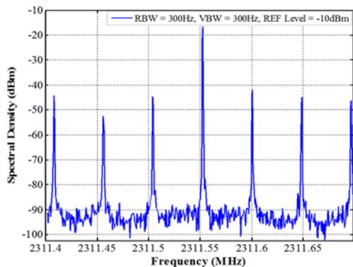
Figure 4: Output signal using 4.2 Km fibre delay line (Span 300 KHz).
