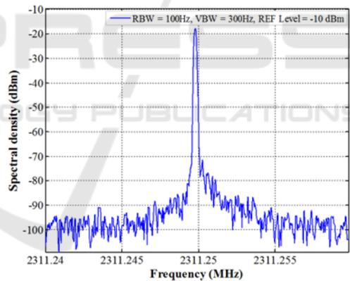
Figure 6: Oscillation mode only using 6.6 Km fibre delay line (Span 20 KHz).
