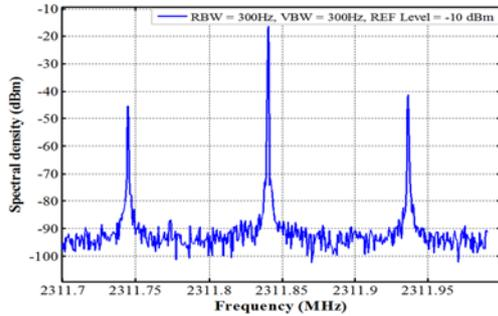
Figure 2: Output signal using 2.1 Km fibre delay line (Span 300 KHz).
