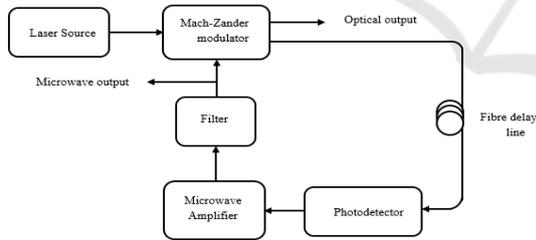
Figure 1: Optoelectronic oscillator structure.
