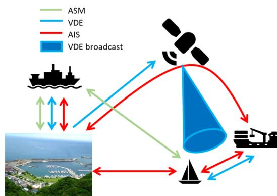
Figure 1: VDES/AIS communication framework.
