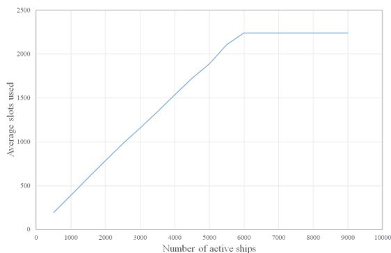
Figure 4: Simulation of AIS messages channel occupation.
