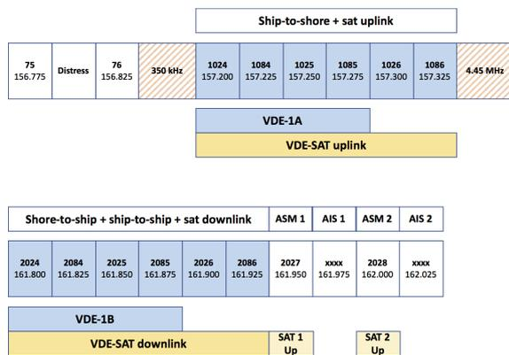
Figure 2: VDES transmission channels.
