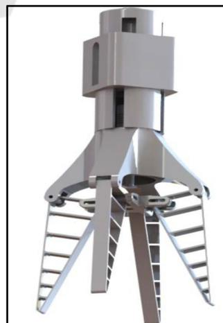
Figure 3: 4-Finger proposed gripper design (Basson, et al., 2017).
