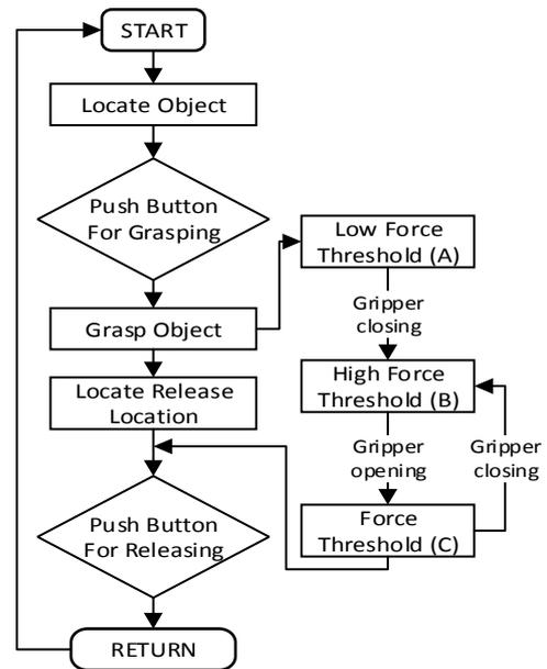
Figure 8: Operational pseudocode for the gripping system.
