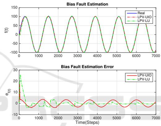
Figure 4: Bias fault and its estimation.
