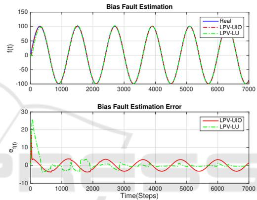
Figure 4: Bias fault and its estimation.
