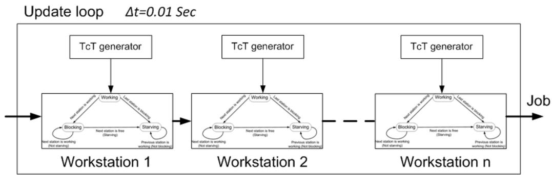
Figure 13: Welding line simulation.
