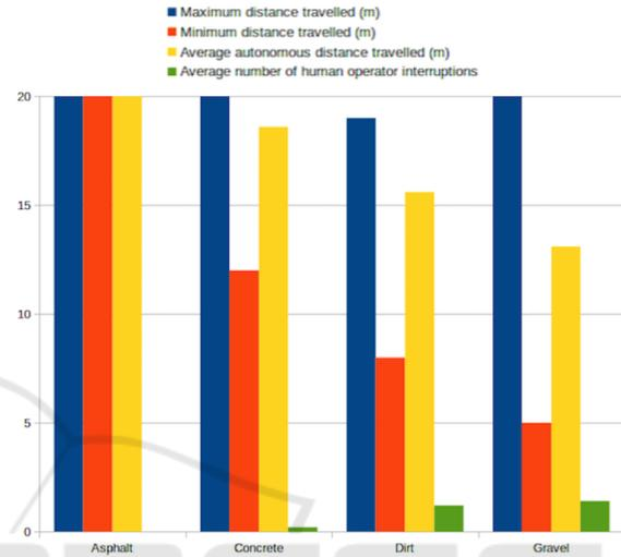
Figure 5: Autonomous test results plot on different trail types (see Table 5 for details). Vertical axis is in meters for distance traveled and count for average number of human operator interruptions.
