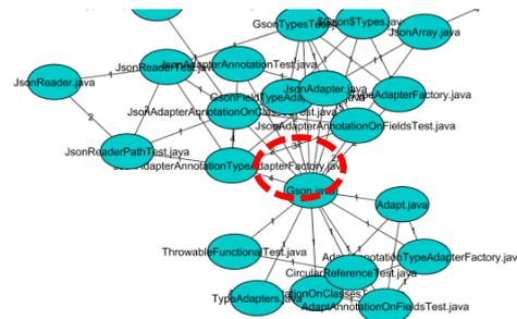
Figure 2: Snippet of Gson project represented in weighted complex network using the proposed method.
