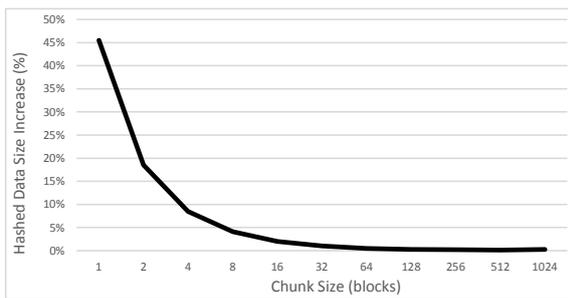
Figure 5: Data Size Increase vs Chunk Size.
