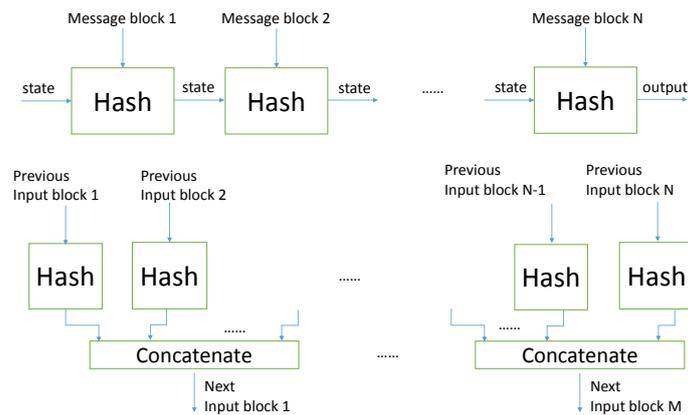
Figure 4: Sequential vs Parallel Hashing.
