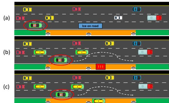
Figure 4: Illustration of the test scenarios for the ‘Dedicated Lane’ case: (a) ‘Low road adhesion due to ice on the road’; (b) ‘Rock falls detected on the road surface’ and ‘Big objects detected on the road’; and (c) ‘Stationary vehicle due to break down’ scenario. The orange color-coded zone indicates the ‘Destination area’.
