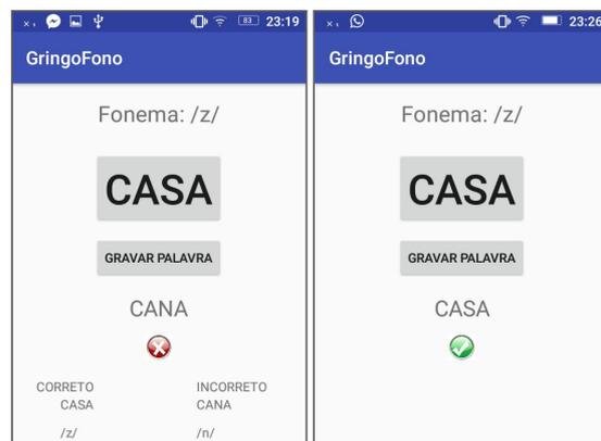
Figure 3: Screenshots of the mobile application performing speech assessments with Google Cloud Speech API (incorrect and correct pronunciation feedback from the word corresponding to the English word "house").
