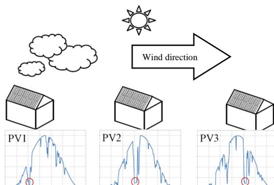
Figure 5: Example of a time-delayed moving power drop at neighbouring PV systems caused by a moving cloud (large images of the PV diagrams in the APPENDIX).
