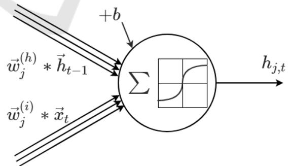
Figure 11: Visualization of the computation in a hidden layer node.  $w$  denote weights,  $b$  bias,  $x$  inputs and  $h$  the hidden layer values.  $j$  is the index of the node in the layer, while  $t$  is the time index.
