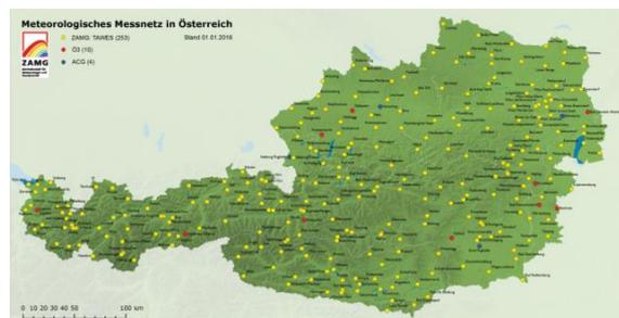
Figure 1: Meteorological network of ZAMG ("Meteorological Network — ZAMG," 2017) which offers meteorological data from more than 250 meteorological stations situated in all climate regions and altitudes Austria-wide.
