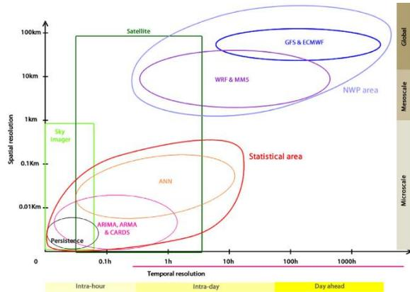
Figure 3: Overview of state of the art forecast methods for PV generation (Antonanzas et al., 2016).
