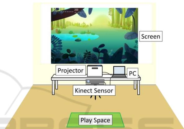
Figure 2: System setup.
