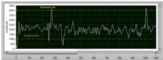
Figure 9: Envelope of the ECG signal (Case Study 1).
