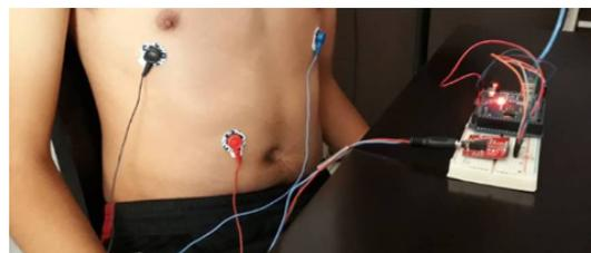
Figure 18: Pad placement and sensor connections (Case Study 3).
