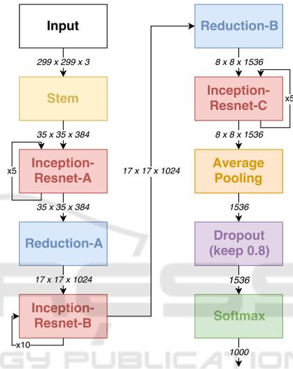
Figure 5: Schema for Inception-ResNet-v2 network.
