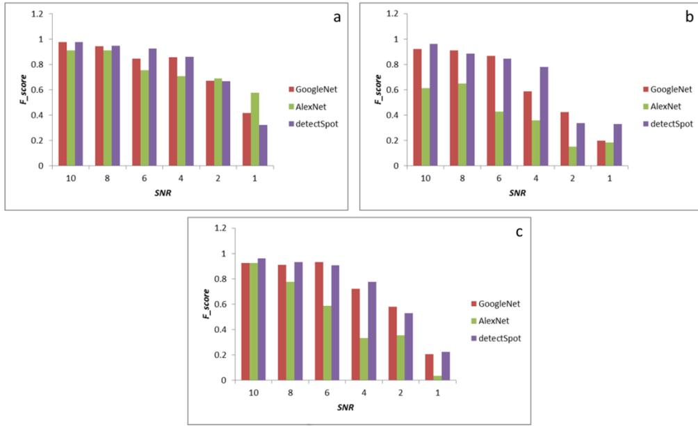
Figure 5:  $F_{score}$  vs SNR curves for all three conv-nets methods applied to two kinds of synthetic images (a) Synthetic type A, and (b-c) Synthetic type B.
