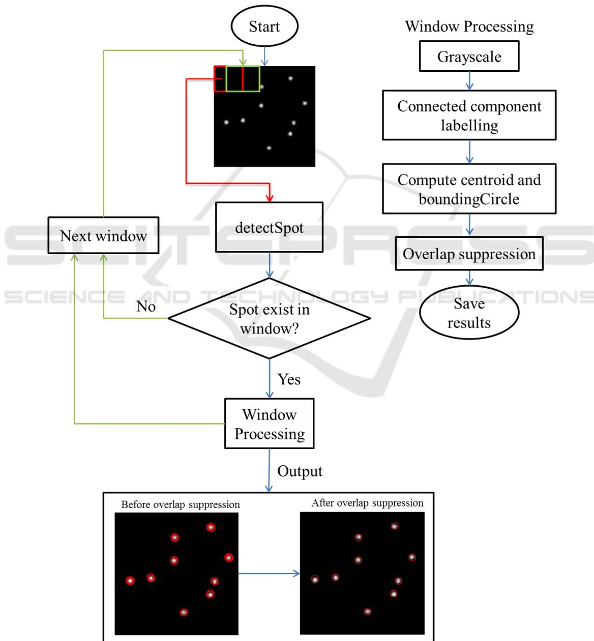
Figure 3: The proposed architecture for spot detection in microscopy images.
