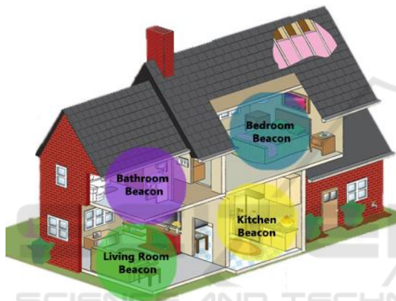
Figure 2: BLE Beacons: Room placement in fictional environment.
