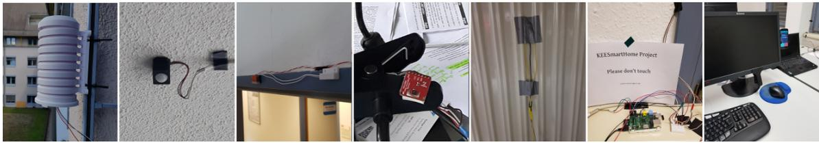
Figure 5: Sensors and UI. Outdoor temperature, motion detection, door, RGB, radiator temperature sensor, Raspberry Pi, and UI (from the left to the right).
