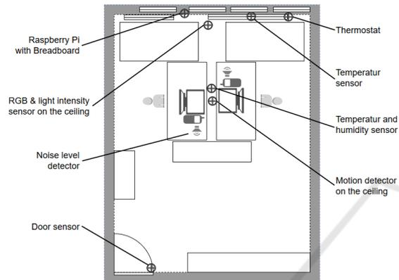
Figure 4: Sensor and HW deployment.
