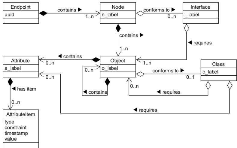
Figure 5: The cloud.iO class model.
