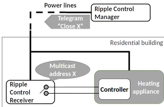
Figure 6: Principle of Ripple Control (RC).
