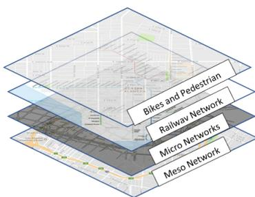
Figure 2: Partitioning the network into different layers.
