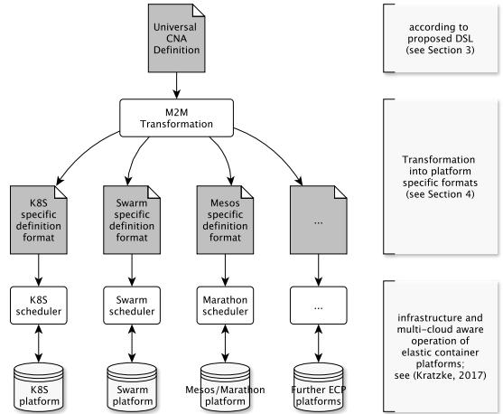
Figure 2: Separation of concerns in deploying a CNA.
