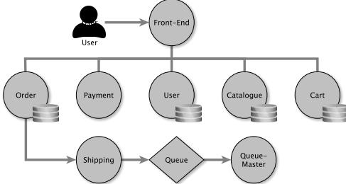
Figure 4: Architecture of the reference application *Sock Shop*, according to (Weaveworks, 2017).
