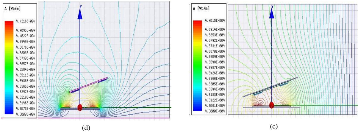
Figure 6: 2-D Magnetic flux distribution between the coupled coils with core. (a) Perfect Alignment, (b) Planar Misalignment, (c) Angular misalignment (d) Planar and angular misalignment (cont.).
