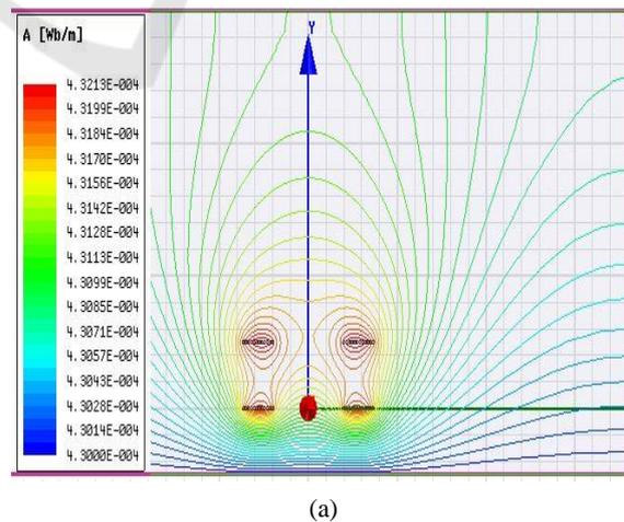
Figure 5: 2-D Magnetic flux distribution between coupled coils Without core (a) Perfect Alignment, (b) Planar Misalignment, (c) Angular misalignment, (d) Planar and angular misalignment.
