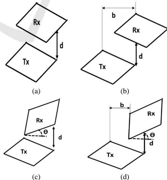
Figure 2: Various misalignment of square inductive coils (a) Perfect Alignment (b) Planar Misalignment, (c) Angular misalignment, (d) Planner and angular misalignment.
