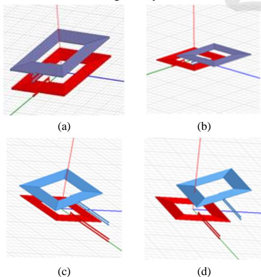
Figure 3: Square Coil arrangement in FEM Simulation (a) Perfect Alignment (b) Planner Misalignment, (c) Angular misalignment, (d) Planner and angular misalignment.
