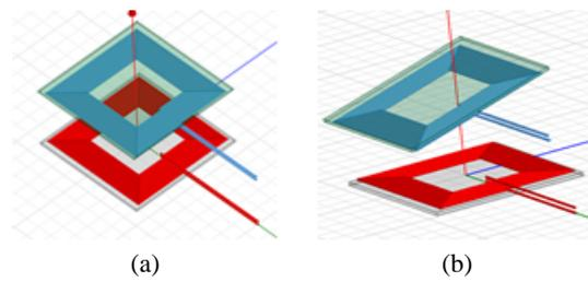
Figure 4: Square Coil arrangement in FEM Simulation (a) Coil setup with Ferrite Core (perfect alignment), (b) Coil setup with Ferrite Core (misalignment).
