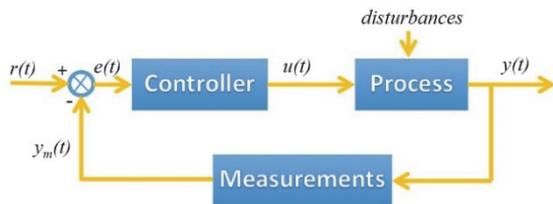
Figure 2: Control diagram in closed loop.
