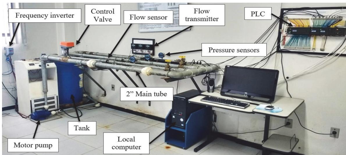
Figure 6: Photograph of the experimental platform.
