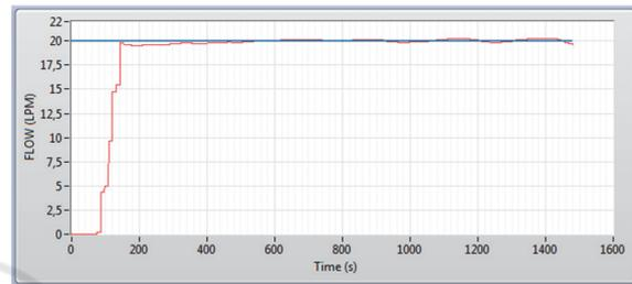
Figure 13: Flow-Current control response.
