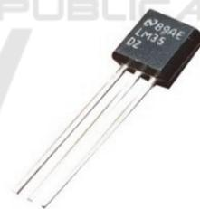
Figure 9: Temperature sensor.
