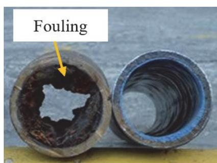
Figure 1: The comparison between tubes with (left) and without (right) fouling.
