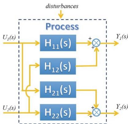
Figure 4: 2x2 MIMO system diagram.
