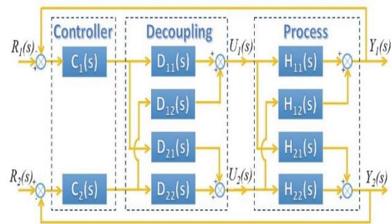
Figure 5: TITO system with decoupling diagram.
