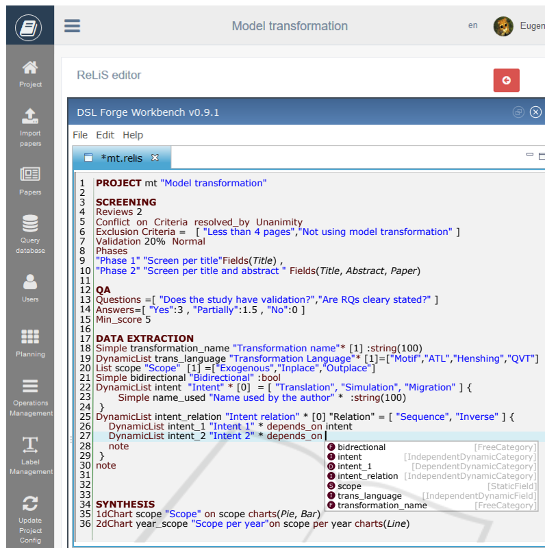
Figure 5: Project configuration model in ReLiS in its textual concrete syntax.
