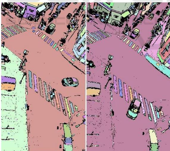
Figure 3: Region extraction and labeling for the reference image and the image to register.
