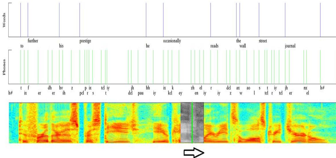
Figure 1: Shows the preparation of the images for GoogLeNet training. A sliding window moves over the 16kHz STFT-based spectrogram. The sliding window is shown in grayscale, the resulting 256\*256 pixel spectrogram patches are placed into phoneme classes according to the TIMIT transcription for training, validation and testing.
