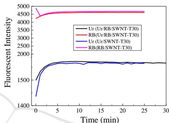
Figure 1: Time-depended fluorescent spectra of **Ur** and **RB** in single-fluorophore(2µL)/SWNT-T30(10µL) system and multi-fluorophore(2µL/2µL)/SWNT-T30(10µL) system, respectively. All the samples were diluted to 2 mL by *Tris* (10 mM). The excitation and emission wavelength was set as 490 nm and 512 nm for Ur, 553 nm and 572 nm for RB, respectively.
