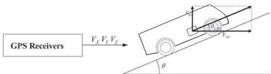
Figure 3: Measuring Road Slope with GPS.
