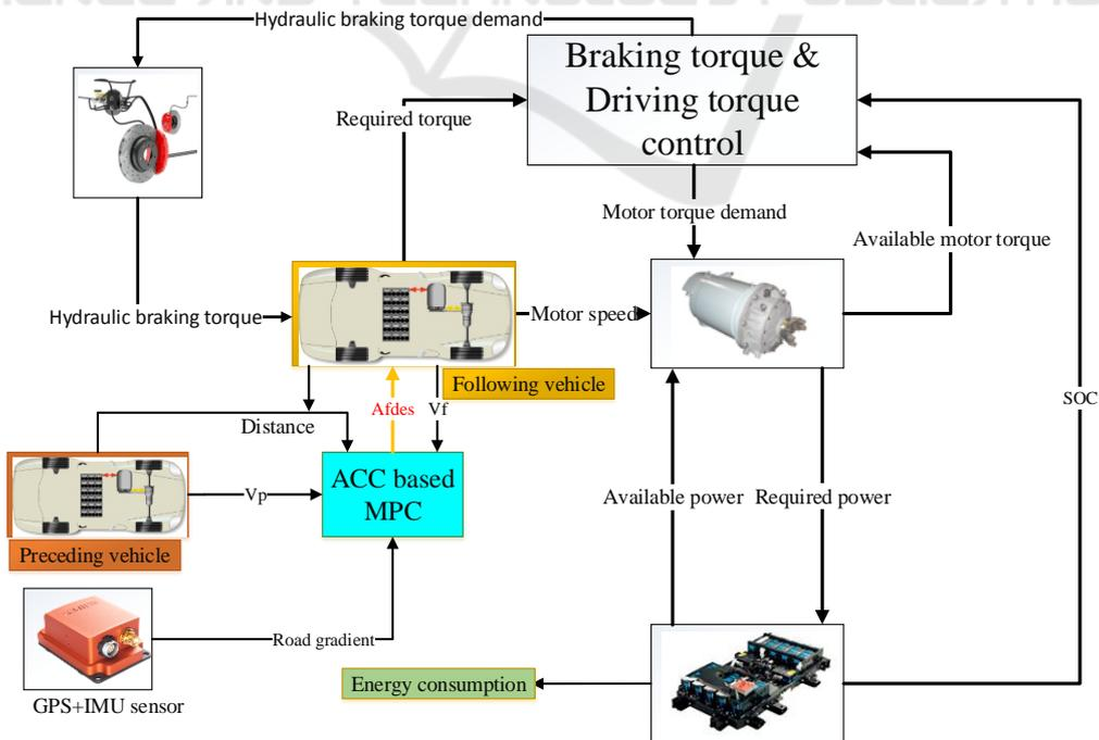
Figure 5: Simulation model.
