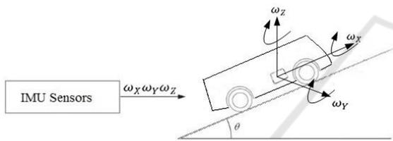
Figure 2: Measuring Road Slope with IMU.
