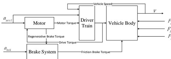
Figure 1: Longitudinal dynamics of electric bus.
