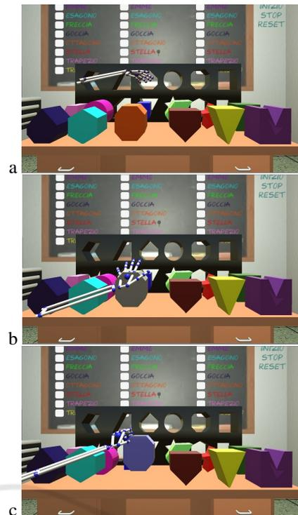
Figure 4: Grasp function: (a) The user looks at the scene (b) The user reaches an object (c) The user grabs an object.
