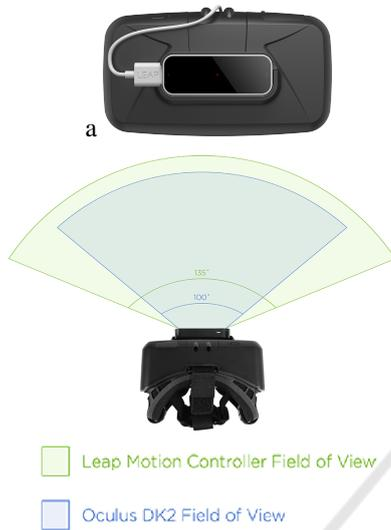
Figure 1: (a) Leap Motion device mounted on the Oculus Rift DK2 (b) FOV of the Oculus Rift and of the Leap Motion device.
