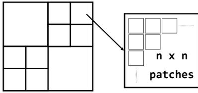
Figure 1: Geometry tiles are selected to honor a predefined screen-space error limit; each tile is subdivided into a fixed number of patches to the GPU.
