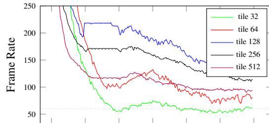
Figure 6: Achieved frame rate along camera path for patch size of  $32 \times 32$ .
