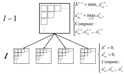
Figure 2: Computed object-space errors: at leaf tiles, for each patch at maximum tessellation level, the associated error is zero; errors are then propagated to other possible tessellation levels. Errors of patches at upper quadtree level are inherited from the lower levels. The error associated to each tile is the maximum annotated to patches at maximum tessellation level.
