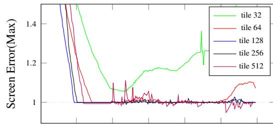
Figure 10: Observed maximum screen space error (in pixels) per frame along camera path (patch  $32 \times 32$ ). Recall we request an error of at most 1 pixel; values above this number signalize the system is not capable of delivering the requested quality in real time.
