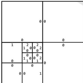
Figure 3: Annotated level differences along tile edges. For each edge of a selected tile, the neighboring tiles are checked; if neighbor tile is at same or higher level, zero is annotated; if neighbor tile is at lower level, level difference is annotated.
