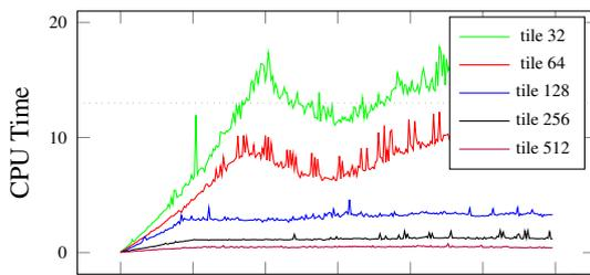
Figure 9: Required CPU processing time (in milliseconds) per frame along camera path (patch  $32 \times 32$ ).
