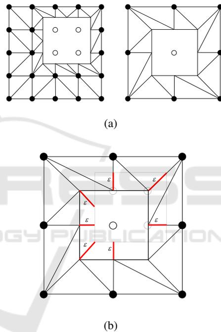
Figure 4: Horizontal object space errors: (a) illustrative patch with void vertices and corresponding coarser level; (b) computed horizontal errors due to border displacement.
