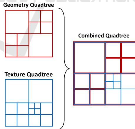
Figure 5: Correspondence among geometry (in red) and texture (in blue) tiles: at the left quadrants, 1-to-1 correspondence cases are configured; at the upper right quadrant, there is a  $n$ -to-1 case and, at the lower right quadrant, there is a 1-to- $n$  case, which requires the use of *virtual geometry tiles* to be rendered.
