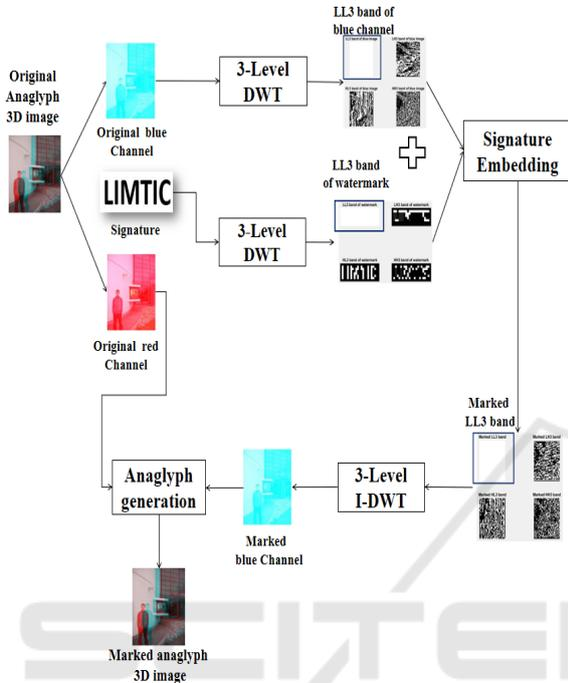
Figure 3: Layout of the embedding process.
