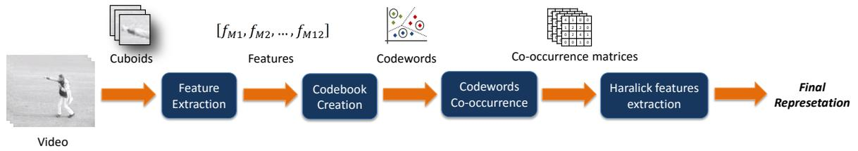
Figure 3: Diagram illustrating the pipeline extraction of the proposed spatiotemporal feature representation.
