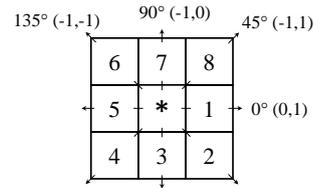
Figure 2: Offset configurations with  $d = 1$ . Cells 1 and 5 are the  $0^\circ$  (horizontal) nearest neighbors to cell \*; cells 2 and 6 are the  $135^\circ$  nearest neighbors; cells 3 and 7 are the  $90^\circ$  nearest neighbors; and cells 4 and 8 are the  $45^\circ$  nearest neighbors to \*. Note this information is purely spatial, and has nothing to do with pixel intensity values (Haralick et al., 1973) (Figure from (Caetano et al., 2016)).
