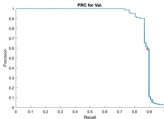
Figure 6: Precision-Recall curve obtained on the validation set at the first stage and used for the operating point selection. Red point identifies the selected operating point.
