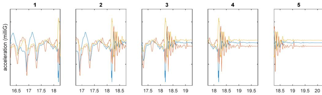
Figure 2: Example of sliding windows with 75% of overlap. Note that only in third and fourth windows the fall peak can be seen entirely. If there was no overlap, only windows one and five would have been considered.
