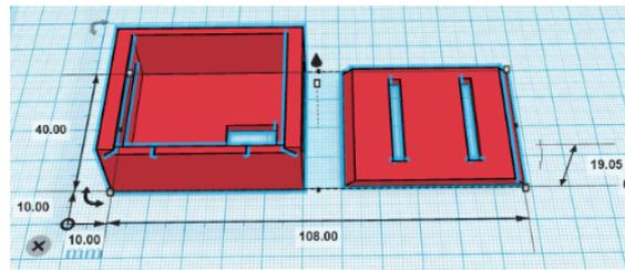
Figure 6: CAD design for the IMU module housing unit, 3d-printed in ABS plastic. Dimensions are provided in mm.
