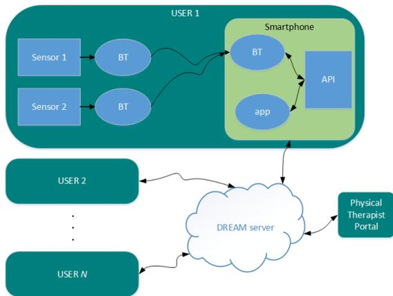
Figure 2: Schematic system diagram of a next generation DREAM exercise monitor.
