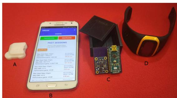
Figure 1: System components of the DREAM exercise monitor: A) Dynofit’s Flexdot wireless EMG sensor; B) the DREAM mobile app; C) the custom packaged wireless IMU board; D) Mio Global’s Alpha 2 heart rate monitor (Mio Global, Vancouver, British Columbia).
