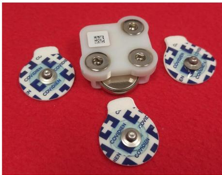
Figure 4: Flexdot components: the plastic housing for the signal processing circuitry, with 3 female snap connections, a 3V-coin cell battery, and the disposable snap electrodes (Medtronic Covidien PLC, Minneapolis, MN).
