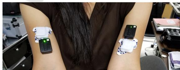
Figure 10: Placement of wireless EMG sensors. Left arm: Trigno sensor placed more proximally, Flexdot sensor more distally. Right arm: Flexdot sensor placed more proximally, Trigno more distally.
