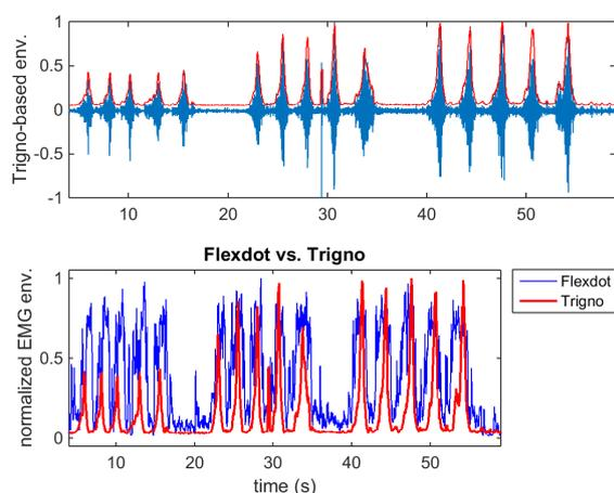
Figure 11: Comparison of Trigno-derived vs. Flexdot-derived EMG envelopes (from left arm) with Trigno sensor more proximal, Flexdot more distal.
