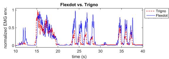
Figure 9: Comparison of EMG envelope acquired from the Dynofit Flexdot by the DREAM app and the EMG envelope obtained from Delsys Trigno.
