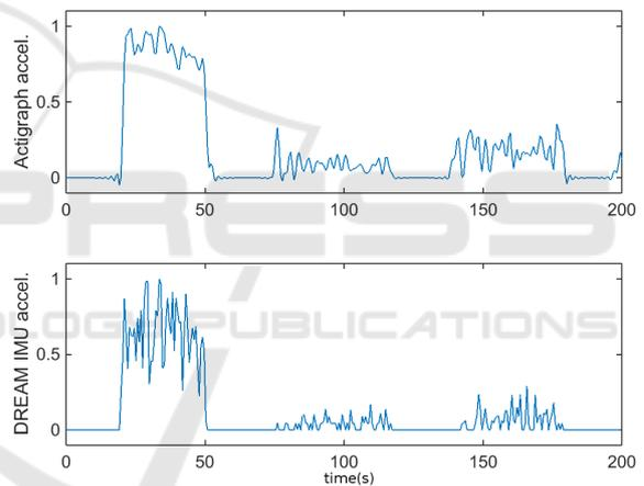
Figure 7: Endpoint acceleration magnitude acquired by Actigraph sensor vs. DREAM IMU module.
