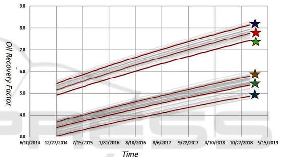
Figure 12: Simulation results of 100 geological models for Oil Recovery Factor.
