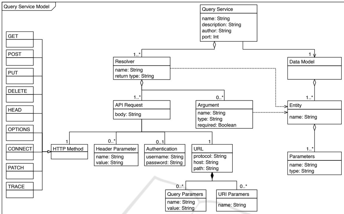
Figure 2: Meta-model of the *Query Service*.
