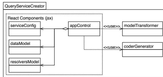
Figure 4: Architecture of the *Query Service* creator tool.
