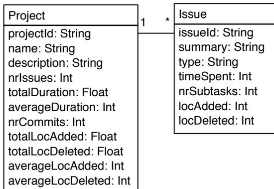
Figure 7: Data model of the example web application.
