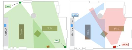
Figure 3: A sketch of the visual sensors fields of view and their overlap. Left panel shows the field of view of the two cameras, while right panel shows the field of view of the two RGB-D sensors.
