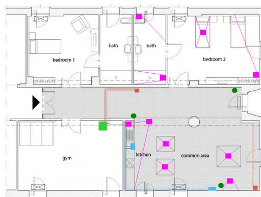
Figure 1: Apartment plan. Blue rectangles represent the RGB-D sensors, the small red squares correspond to the cameras. Green circles represent the localisation tags, while purple rectangles indicate the Passive Infra-red (PIR) sensors and their field of view (through purple lines). They are all wired to the workstation (green square), placed in the gym.
