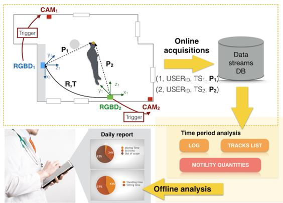
Figure 4: A visual sketch of the pipeline of our system. Video acquisition is triggered by the RGB-D depth sensors which detect the presence of individuals in the common room. Acquired data are stored online in a Data Base that makes data available for offline analysis.
