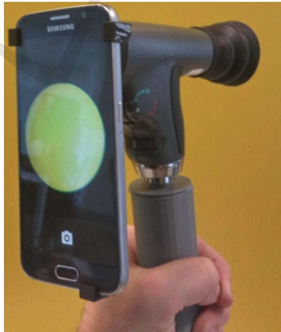
Figure 1: Assembled EyeFundusScope prototype.
