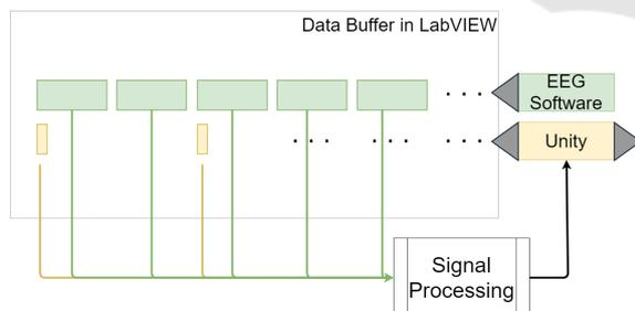
Figure 3: Streaming protocols. EEG data is streamed from the EEG software to LabVIEW in buffer times of 20 or 50 ms. The game engine streams events directly to LabVIEW. Data is immediately sent to the signal processing thread in LabVIEW and feedback is sent back to the game engine.
