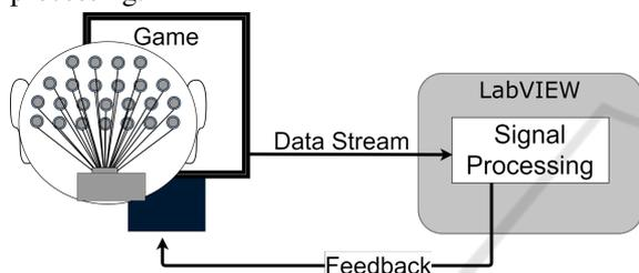
Figure 1: Overview of the future experimental setup. A subject is placed in front of a computer screen. EEG data is recorded simultaneously as the subject is performing a computer task. EEG data is continuously streamed in real time to LabVIEW for signal processing. Feedback from the recorded EEG data (visual and/or tactile) is then provided back to the subject.
