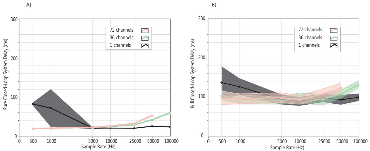
Figure 5: (A) Pure closed-loop system delay. Median system delay with associated median absolute deviations across measurements ( $n=50$ ) are shown as a function of sampling rate (Hz) for streaming with 1 channel (black), 36 channels (green), and 72 channels (pink). (B) Full closed-loop system delay. Same as in (A).
