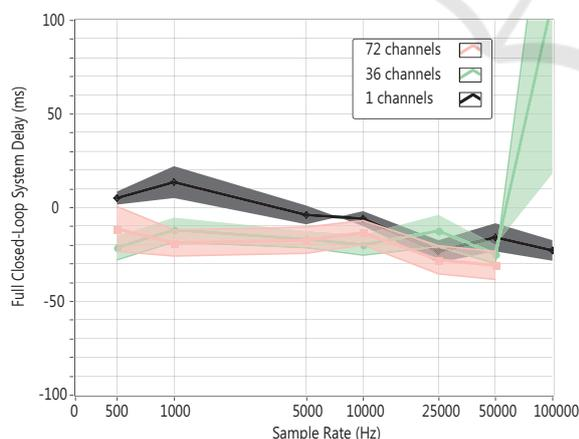
Figure 7: Effects on the full closed-loop system delay by using a PyCorder buffer time of 20 ms. The full closed-loop system delay using a buffer time of 50ms is subtracted from the full closed-loop system delay using a buffer time of 20ms. The median difference is shown with associated median absolute deviations across measurements (n=50) as a function of different sampling rates (Hz) for streaming with 1 channel (black), 36 channels (green), and 72 channels (pink).
