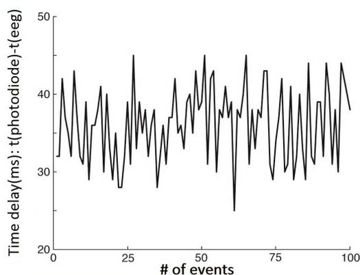
Figure 4: Visual presentation delay. The delay between the timestamp of the EEG input trigger (the game engine sends a trigger to the EEG via a parallel port) and the presentation of a visual stimulus on the screen, as detected by the photodiode, is shown for all measurements (n=100).
