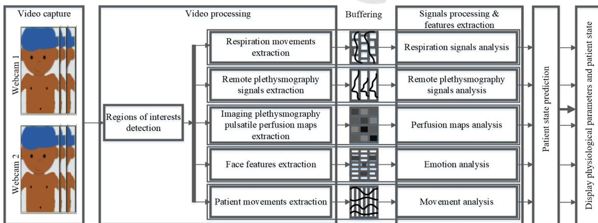
Figure 1: Block diagram of system architecture.
