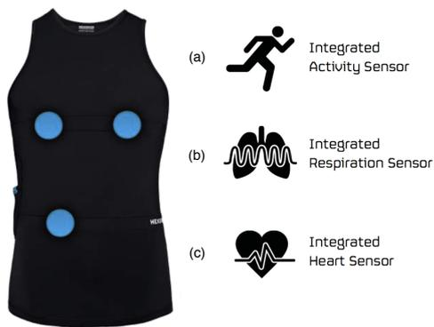
Figure 1: The Hexoskin acquisition system: (a) Activity sensor, (b) Respiration sensor and (c) Heart sensor.
