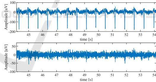
Figure 7: From top to bottom: 5 Hz high-pass filtered signal and RLS adaptive filtered signal.
