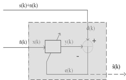
Figure 4: Typical scheme of an adaptive noise canceler.
