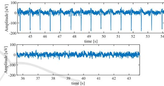
Figure 6: From top to bottom: 5 Hz high-pass filtered signal and processed signal by QRS blanking.
