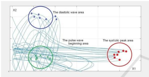
Figure 5: The example of main point selection for the rheocardiographic signal – the projection of the rheocardiographic signal portrait on the X1 and X2 axis.
